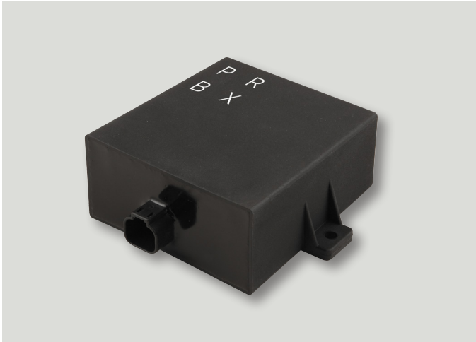
Rugged DC/DC Booster for Marine diesels engine delivering constant voltage to the engine monitoring system during startup. The unit generates boosted voltage to compensate lower battery voltage during the ignition phase.
