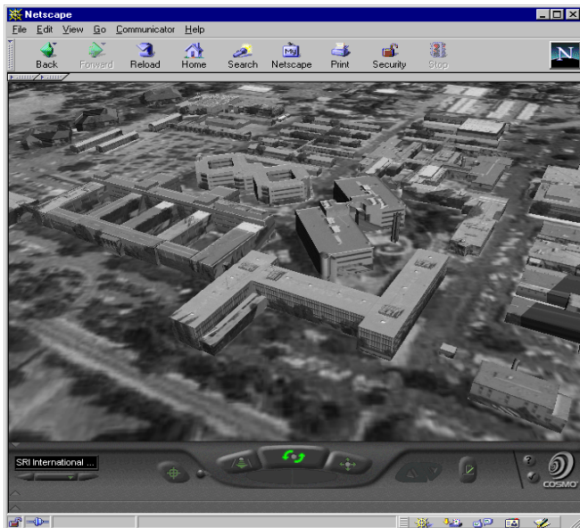
Figure 10. A texture-mapped site model of the SRI International campus that has been georeferenced onto an underlying terrain model. Note the accurate alignment of the latitude/longitude-specified buildings with the underlying 1 m resolution USGS DOQ satellite imagery in UTM coordinates.
