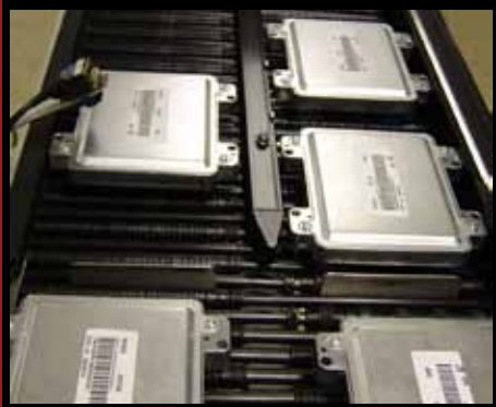
Automotive Electronics Assembly and Test System using Bi-directional Flow with One Frame and One Drive
