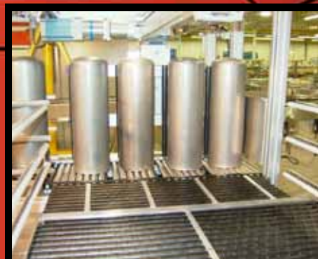
Pattern Forming and Indexing using Right Angle Transfers to feed Single or Multi-product Processes
