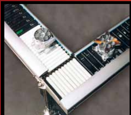
Tight Right Angle Transfer with Traffic Control
