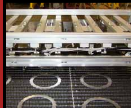
Multi-lane Conveyance of Metal Parts during Cooling Process
