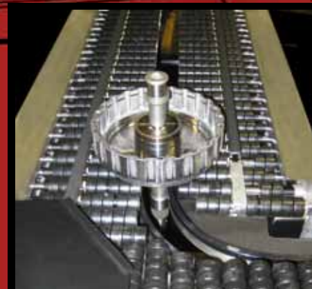
Open Center Track System with Customized Conveyor Surface
