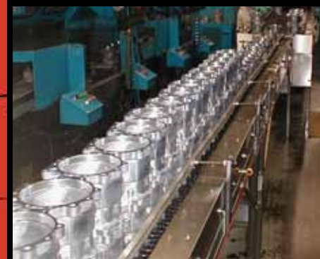
Precision Machined Edges are Protected with Slip-torque Slip-fit Technology to Buffer the Product and Increase Efficiency
