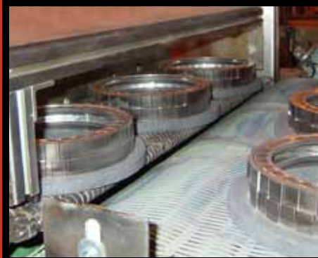
Extended Roller Transfer of Powdered Metal Parts Eliminates the Need for Dead Plates
