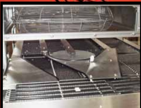
Serpentine Cooling with Bi-directional Product Flow
