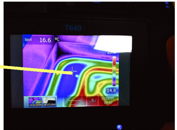
Drilling test holes (for % moisture) between underfloor heating pipes under rubber floor
