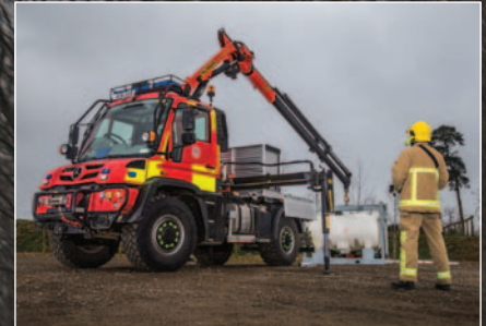
1,500-litre water tank with pump and hose reel.
