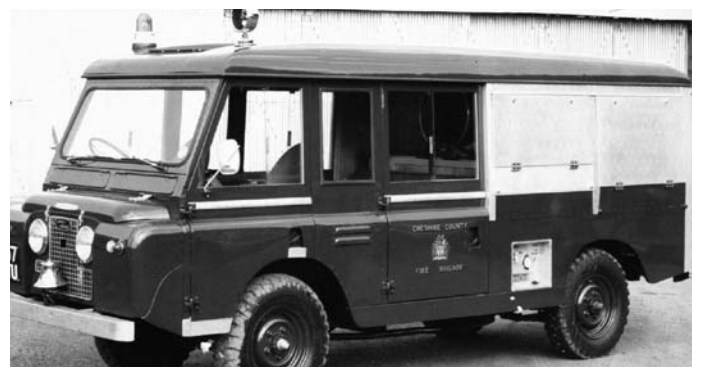
Away from major pumps, this 1970 image captures Cheshire County Fire Brigade's new Land Rover L4P forward control rural light pump.
