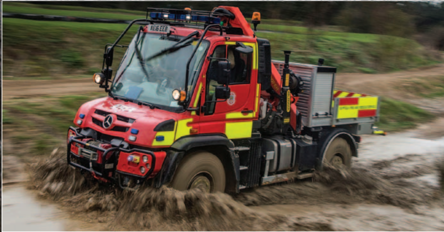
1,500-litre water tank with pump and hose reel.
