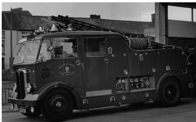
Another classic fire engine seen in post-war fire brigades was the AEC Regent. This 1960 view is of a Merthyr Tydfil Fire Brigade pump escape running with a 50ft all-metal Merryweather ladder.
