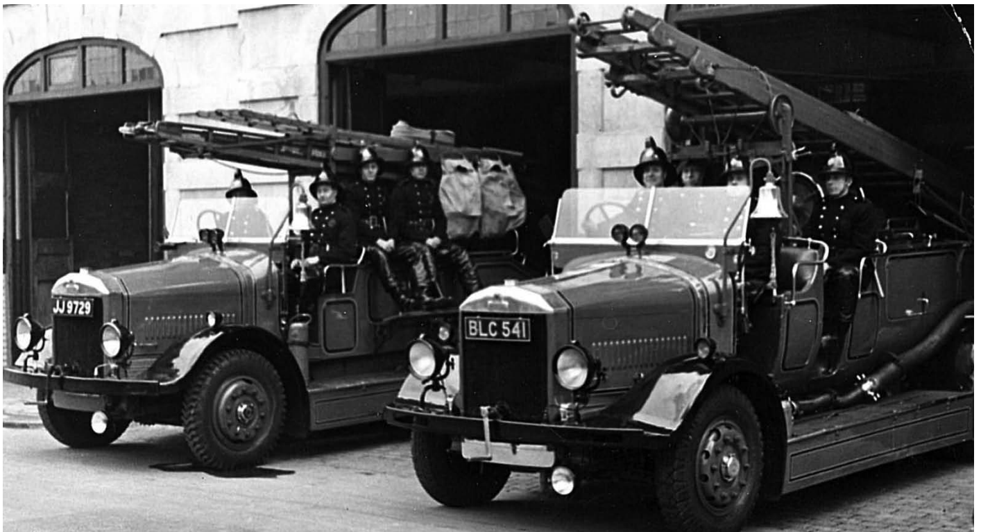
Two London Fire Brigade Dennis Big 4s pictured in 1948 at Redcross Street Fire Station in the Barbican area of the City. The pump on the left is a 1933 model with lateral side seating. Note the two Proto oxygen BA sets hanging behind the nearside crew, whilst the pump escape is a 1935 version with transverse seating for the crew. Redcross Street was right in the heart of the worst WW2 Blitz period but both pumps survived the war years and were retired in 1955. (Image from Neil Wallington's collection.)
