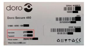
The setup username and password are printed onto the label's left hand side (red box in above picture).
