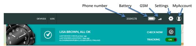
The settings icon can be used to access the setting page. The My Account icon can be used to access My Account settings, Geofences (if user has access rights to create and edit geofences) and to Log out from the Doro Secure 480 web service.
