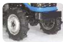
4WD FRONT AXLE (For better traction. Suitable for muddy opration better steering angle for sharp turning)
