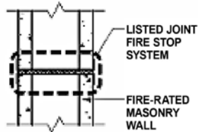
Figure 5.8: Joint Fire Stop System in Movement Joint Between Adjacent Masonry Walls (Ref. 2)
