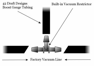
Tubing must be installed as shown!
