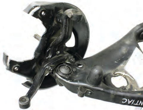
Lower Ball Joint Installs from the bottom, facing down
