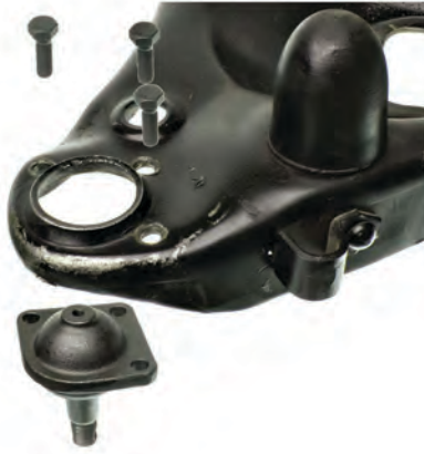
Lower Ball Joint Installs from the bottom, facing down
