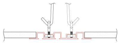
fixing 4560 in suspended ceiling with 4555-SH
