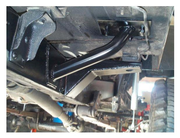
Once those are cut, setting them into a place that will connect with the bars selected for each mount, tire size and suspension movement is critical for each placement.
