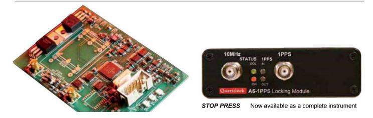
This is a PCB level product to control an OCXO or Rubidium oscillator from an external 1PPS. The A6-1PPS uses a 3 state Kalman filter algorithm to measure & correct the frequency offset of the oscillator with respect to the 1PPS input. Time-tagged 1PPS to 200ps resolution & <1ns jitter.
