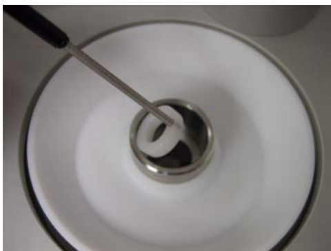
Figure 7. Replacing the reference cell lid over the reference cell port.
