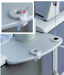
Figure 5. Sample tube in place in the holder. The lid of the sample tube fits into the groove in the holder (marked with an arrow in the inset).
