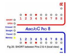
8. Press the TEST button to proceed, if there are more failures the test will stop at each and everyone of them, finally only the FAILED and MEMORY LED's will be ON.To test another cable repeat steps 3 & 4. To clear the MEMORY option either, switch OFF and then ON again or, press and hold the test button until the MEMORY LED goes OFF.
