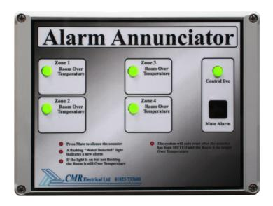
The AS4 Alarm Annunciator has been designed to advise operators or security staff of any plant room or environmental faults. The unit has four independent zones and can interface to any plant containing volt free alarm or fault contacts such as air conditioning plant, water detection systems, generators or UPS systems.
