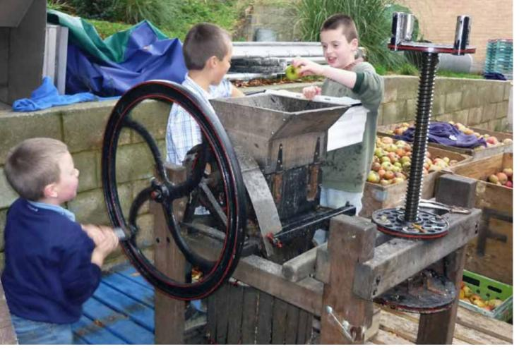
Technology for children should help them understand mechanical properties and forces, whether simple – using a saw to cut wood – or complex. Using a cider press, children experience how their physical effort turning the crank rotates the shaft that chops the apples; then when they screw the press onto the chipped apples, they see the juice flow out the bottom – a clear progression of cause and effect.
