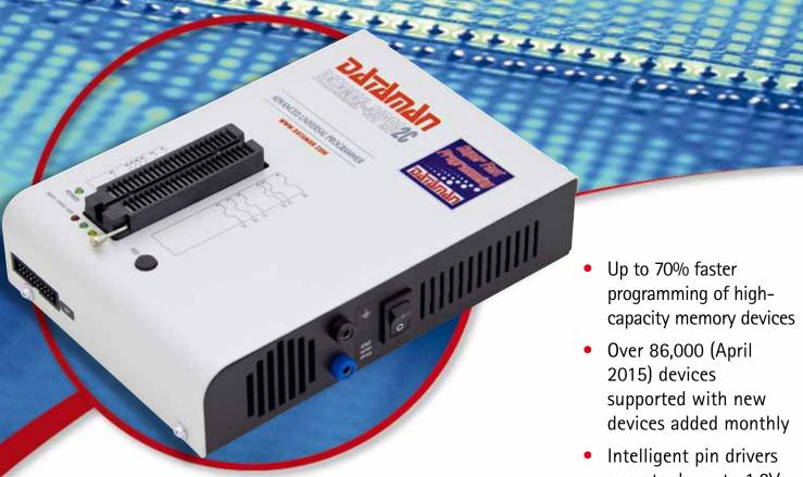
The Dataman 48Pro2C is a super fast PC based universal 48-pin programmer with ISP capabilities and USB 2.0 connectivity. The 48Pro2C is built to meet the demands of development labs and field engineers for super fast universal programming.
