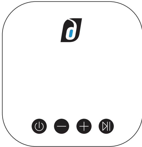
Power/Mode (BT/Aux/JSN), Vol -, Vol +, Play/Pause.
