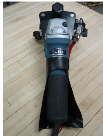
FIGURE 7 – Spray Skirt Installation Complete
