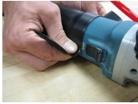
FIGURE 5 – Spray Skirt Installation
