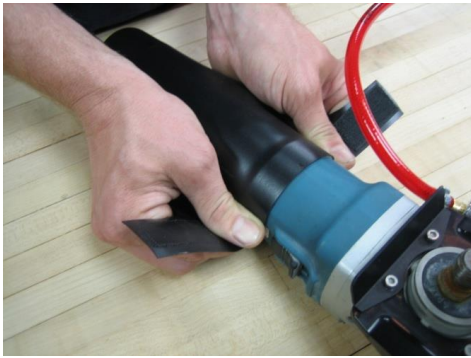
FIGURE 4 – Spray Skirt Installation
