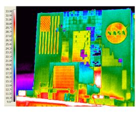
cooler, also were apparent. A visual check clearly showed these to be sections of the building that had been damaged by last year's hurricanes and were in the process of being repaired.
