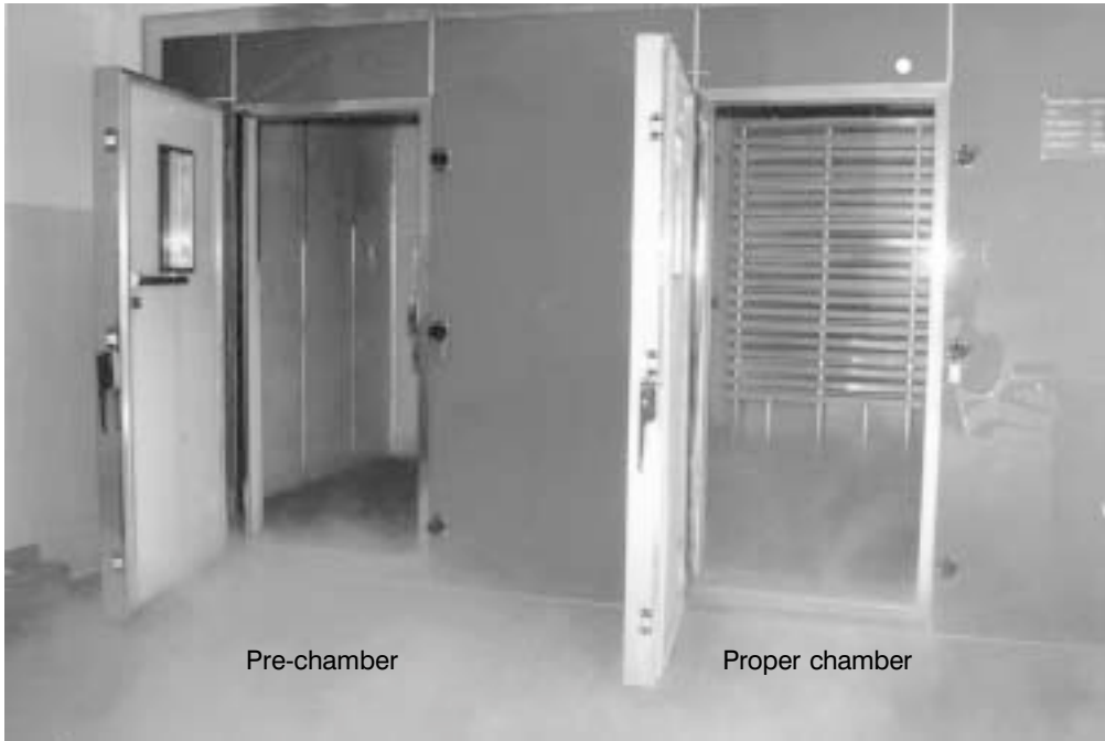
Fig. 22. Picture of a low-temperature cryochamber „Wroclaw type“.
