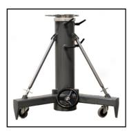
The tripod is adjustable in height (range 900-1400mm) and the weight of the tripod column is balanced by a gas spring. A side handle allows for vertical and horizontal movement of the tripod. A removable and rotary shelf allows positioning of the laptop next to the measuring arm.
