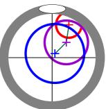
Diagram two: Representation of the rings and bubble as they would appear on the film with added centres crosses and green line showing deviation of borehole.
