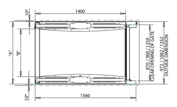
CLEARANCE EITHER SIDE OF STEPLIFT MUST BE <10mm OR >150mm TO COMPLY WITH BS6440.
