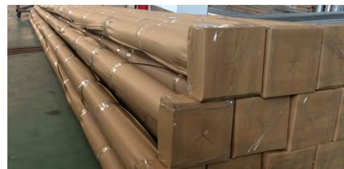
Eran Industrial uses reinforcement nylon bags, bubble bags and corrugated packaging multilayer light poles, three layers of packaging can be carefully protected to ensure the lamp post, lamp post not to be damaged in transportation.
