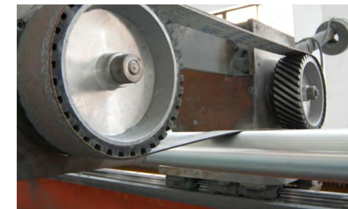
Through large full CNC spinning equipment, raw materials are made into conical or profiled bar in the process of high speed spinning. All the poles do not allow longitudinal welding line, and it requires smooth lines and excellent roundness.
