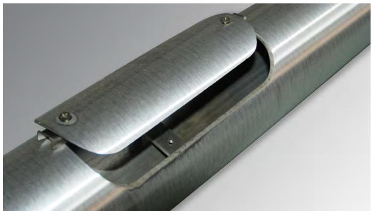
Each pole has a junction box for electric door installation. Eran Industrial adopts advanced cutting equipment to cut the hole door, the door becomes a part of the rod body, ensuring the waterproof of electric door. We use Allen key to protect the door, mean time we welding workpiece "L" for the grounding wire.
