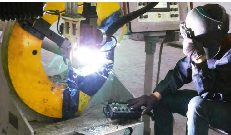
The base uses A356 low pressure casting, and T6 heat treatment, we use automatic welding equipment to connect base and pole. The welding quality has the Canadian welding Bureau certification. In this high quality welding process, the welding strength and beauty are guaranteed.
