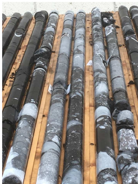
Figure 32: Breccia / Conglomerate within the Upper Dark Limestones (N02748, 421-427m) (NQ – diametre core, 46.7mm)
