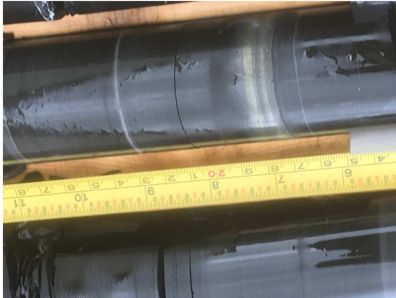
Figure 33: Fine grained pyrite, replacing coarse grained beds / laminae (Drillhole N02748, 417m)
