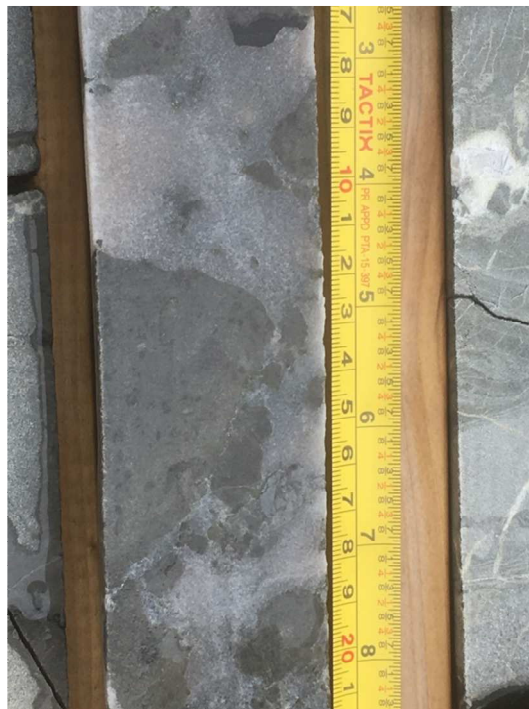
Figure 35: Micrite Unit, Brecciated, disseminated sphalerite and evaporites (Drillhole N02748, (1193m)
