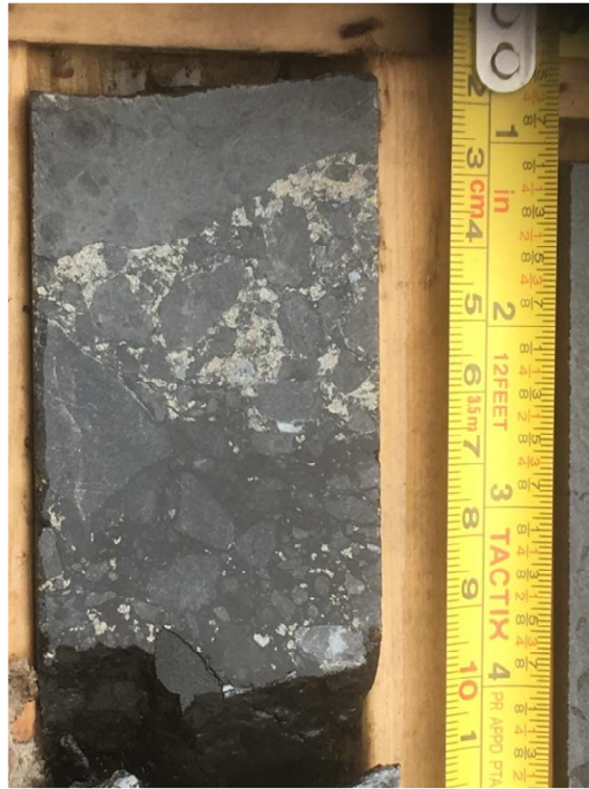
Figure 34: Sphalerite mineralisation in brecciated Navan Beds (Drillhole N02748, 1178m)
