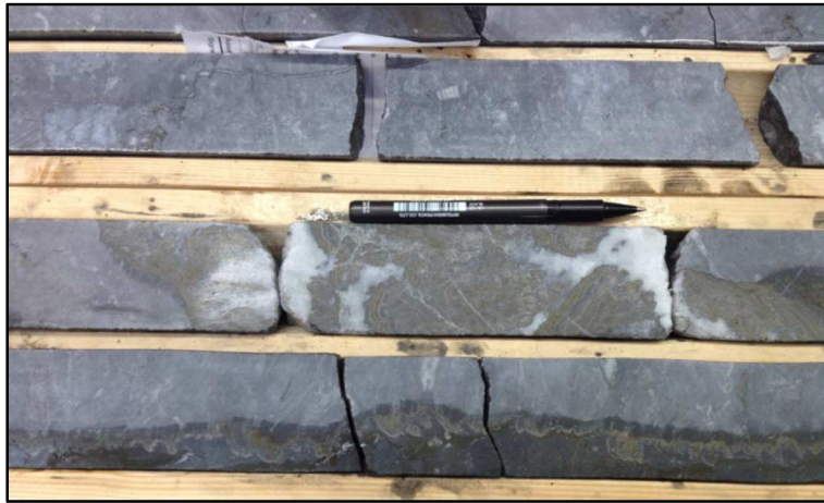
Figure 37: Cavity fill sphalerite-pyrite (Sample D17137 - 262.3-263.3m) in Waulsortian Limestone - drill-hole 3470/11 Ballymoney Bridge.
