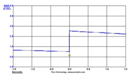
Peak pressures achieved ranged from 1.4 to 2.6 BAR with the vent blades free to open. This is for Propane only. Acetylene and oxygen mix max pressures to be added at a later date. Maximum pressure calculated for propane air mix with no venting would be 6.8 BAR.
