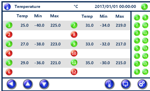
12 Channel display with 16 relays
