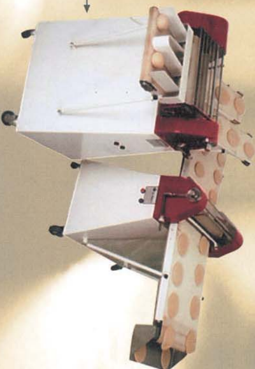
Flattening machines with adjustable rollers for the flat bread sizes control
