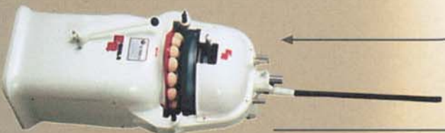
Manual divider rounder 40 to 120 gr' per bowl
