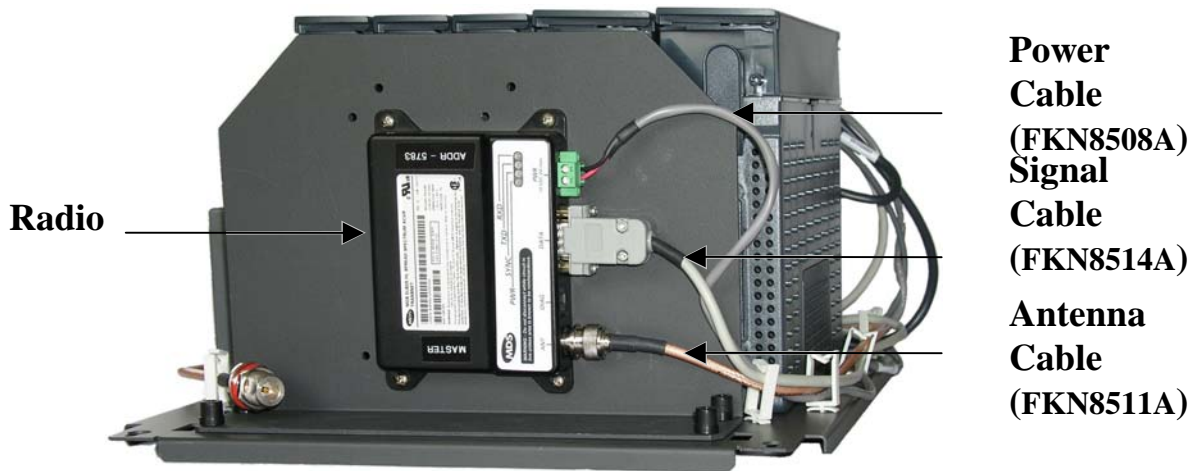
Figure 13-43 TransNET 900 Radio Modem Installed on ACE3600 Chassis – Cable Connections
