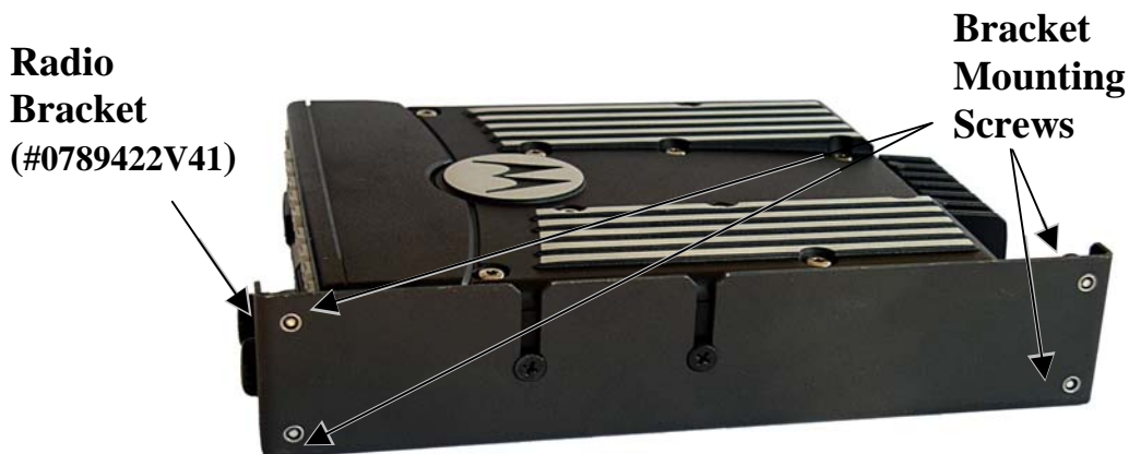
Figure 13-3 XTL5000/XTL2500 Radio Bracket with Four Bracket Mounting Screws
