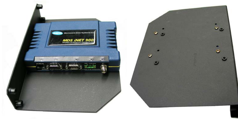
Figure 13-46 iNET 900 Radio Modem Mounted on Metal Bracket – Front and Rear View
