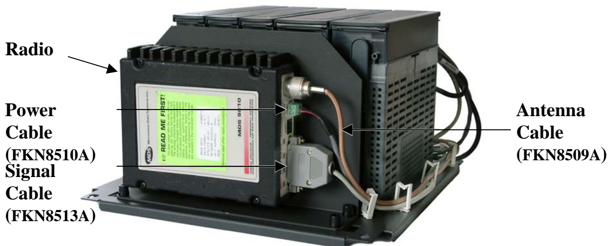
Figure 13-54 MDS Radio Modem Installed on ACE3600 Chassis – Cable Connections
