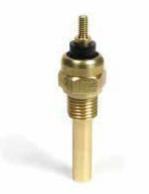
This probe incorporates a resistive bulb that is insulated from the brass body. The sensing wire is wrapped around an insulating mandrel or core and one end of the wire is grounded to the body. Temperatures are measured over a one inch section of the probe. This probe is currently used in tens of thousands of aircraft.
