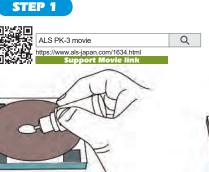
Prepare the glass plate, and put a few drops of polishing diamond on diamond polishing pad.
