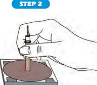
Hold the CV electrode at right angle to the pad.
