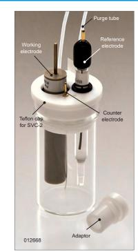
Working electrode and reference electrode are sold separately. Each component could be purchased separately. For acquisition separately, the sample vial of 20 mL is composed for 10 pieces
