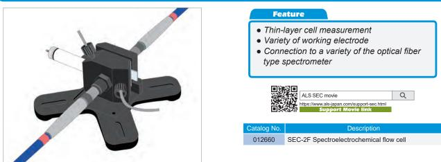
Using the spectroelectrochemical flow cell, it is possible to have different optical path length by changing the gasket. We offer, as an optional item, a silicon and Teflon gasket with 100, 250 and 500  $\mu$ m of the thickness. Flow injection analysis or stopped flow analysis with thin layer cells which was impossible with SEC-C Thin Layer Quartz Glass Spectroelectrochemical cell kit became possible.
