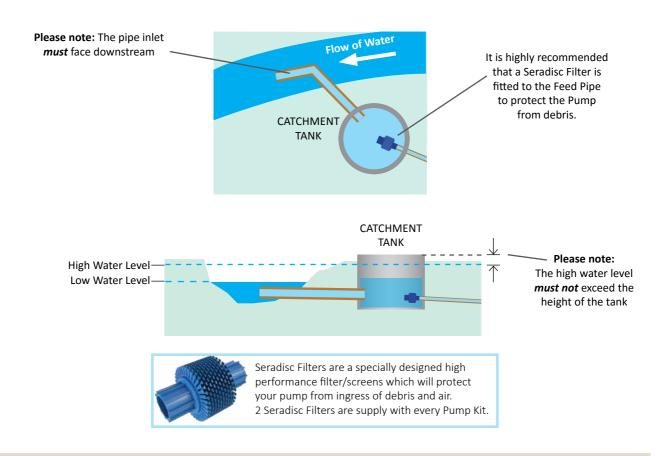
Recommended Pipe for Inlet Pipe and Feed Pipe: **110mm Soil Pipe** (up to 2 pumps) or **150mm Soil Pipe** (3+ pumps)
