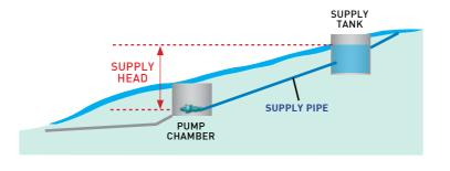
If the Spring/Stream is on a steep gradient you can achieve a good Supply Head within a small distance. In this case, water can be fed directly to the Supply Tank.
