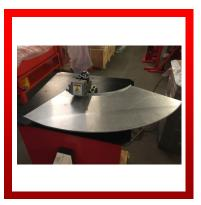
WNS 16swg (1.6mm) POWER FLANGERS are principally used for forming a right angle flange on curved, straight and irregular shapes. These machines are fitted with a tilting head to enable complete circles to be formed. WNS Power Flangers are manufactured with hardened top plates, shafts, forming rolls, gears and guide fences.
