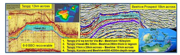
The Beehive prospect is a Carboniferous age 180km² isolated carbonate build up with 400m of mapped vertical relief, analogous to the giant Tengiz field in the Caspian Basin. It is located in 40m water depth suitable for a jack up rig, within ~75km of shore and developable by either FPSO or pipeline to existing infrastructure. This play type is new and undrilled in the Bonaparte Basin with no wells having been drilled to this depth in the basin.
