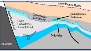
In 2017, Melbana undertook a reprocessing and inversion study of selected seismic lines across the Beehive Prospect with very encouraging results. The seismic inversion results combined with the results of the reprocessing have enhanced the understanding of the Beehive reservoir and seal units.
