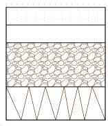
38-40mm Grass Reinforcement Grid 40mm sand/ loam root zone Geo-textile Layer
