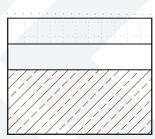
38-40mm Grass Reinforcement Grid 40mm sand/ loam root zone Geo-textile Layer
