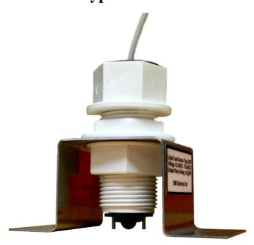
The sensor has been designed to detect the presents of oil or any non-conductive liquid including fuel oil, diesel etc. and energise an internal relay to provide a signal to existing alarm systems, Building Management Systems or SMS messaging systems.
