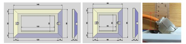
By using these new components, the minimum recommended back box depth is now only 35mm (see image above); giving greater flexibility during installation and maintaining the mechanical and electrical performance of the cabling system.
