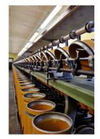
Twisting machine where we inclose individual fibers even more and upgrade the yarn
