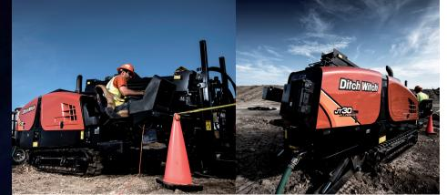
You asked for a drill that tackles the toughest conditions, from solid rock to cobble and hard dirt. You wanted a compact design to operate in the tightest spots. You needed a patented, inner-rod design to save you time, and a mechanical drive to save you money on drilling fluid and transporting water.
