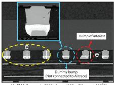
No EM failure up to 7000+ hours (650 miliAmps at 160°C)
