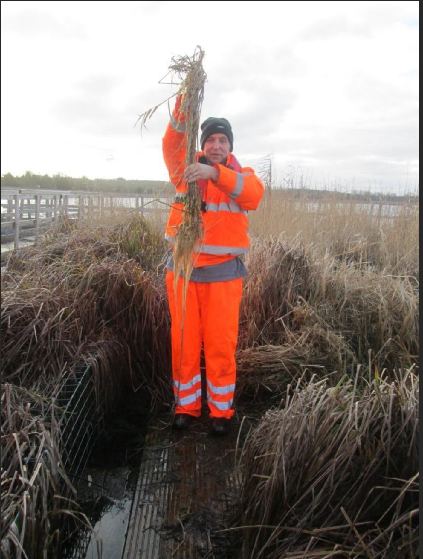
The Living Filter designer & fabricator - plant and internal matrix samples being removed to determine plant health, root biomass (to 1.6m depth) and root colonisation of beneficial microbes – laboratory DNA finger printing is undertaken for accurate species identification.
