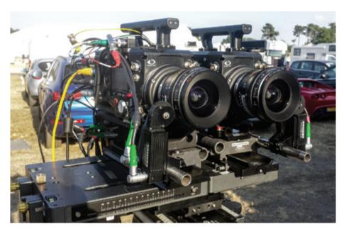
The two matched Flex4Ks in a side-by-side stereo rig.
