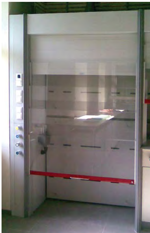
Drive-in cupboard with side control panel
