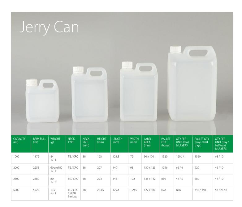
Manufactured in high density polyethylene, available in 4 sizes - 5 litre, 2.5 litre, 2 litre & 1 litre.
