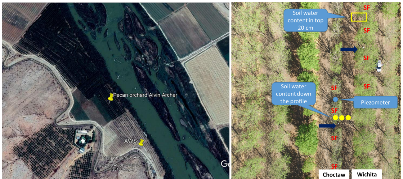
Figure 2: Location of the study site in the Groblershoop region and the experimental layout in the mature pecan orchard. SF indicates the trees in which sap flow is measured. The yellow rectangle indicates where the soil water content of the topsoil is measured. The yellow dots indicate where soil water content down the profile is measured. The blue dot indicates the location of the piezometer for determining the level of the water table.
