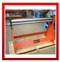
WNS INITIAL PINCH HAND BENDING ROLLS (BR1300/75wns) are principally used for rolling tubes/cylinders in sheet metal. The metal is 'pinched' between two rolls and curves as it comes into contact with the third (back) forming roll. The BR1300/75wns has a 1300mm Roll Length, 75mm Roll Diameter and can accommodate Mild Steel up to 1.5mm thick. The rolls are bottom slip, with an Edwards Style fabricated steel frame.
