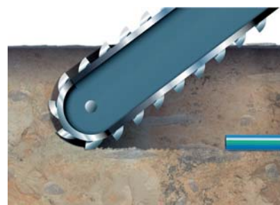
Fig 4-3: Special equipment cuts a narrow pipe trench into which the flexible pipe is laid in the same operation. The excavated soil is used as backfilling material.
