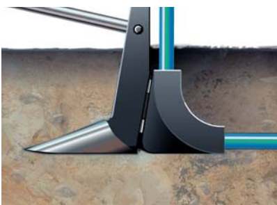
Fig 4-2: In this procedure, the new pipe is ploughed in continuously, and the pipe furrow is closed again immediately afterwards.
