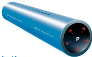
Fig 4-5: Notch test (ISO 13479)
