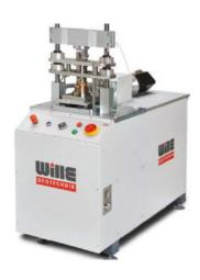
This is advanced fully an simple-shear automatic apparatus with two high quality servomotor drives for static, cyclic and dynamic shear loads up to 10kN. It has a sophisticated robust construction connection with high-quality mechanic and electronic components and includes of a high stiffness frame and actuator system to compensate deformation in static or cyclic loading.
